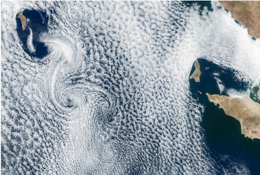
Fig. 12-36. Vortices in the stratocumulus cloud field trace von Kármán vortices downwind of Guadalupe Island, 24 May 2017. NASA Landsat.
