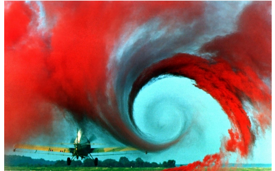
Fig. 10-7. A wingtip vortex revealed by smoke. NASA EL-1996-00130
