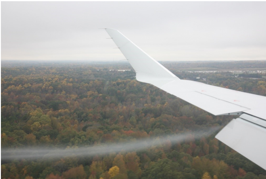
Fig. 10-4. Contrail behind aileron with stratus over NJ 04 Nov 2015 . SDG.
